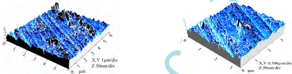
(a) Vibration parallel to the speed of wheel (b) Vibration normal to the speed of wheel Fig.8 The 3D plot of the ultrasonic ductile grinding surface with different direction ( a_p=5\mu\text{m} )
