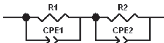
Fig. 8. Equivalent circuit of the 150 nm thickness ZrO_2 thin films humidity sensor.
