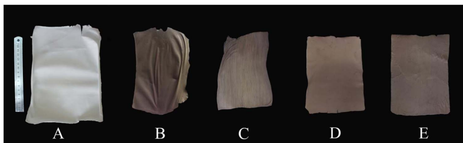
Fig. 9. Digital photos of the UFPPMs prepared using different heating rates of (B) 15 °C/min, (C) 10 °C/min, (D) 5 °C/min, and (E) 1 °C/min. The sintering temperature was 380 °C and the nascent membrane is shown in (A)..
